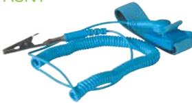
The wrist strap is the most common and effective means of protecting electronic devices from generated ESD. It is made from high-comfort-factor fabric and includes an extendible coiled cord fitted with  $1M\Omega$  resistor.
