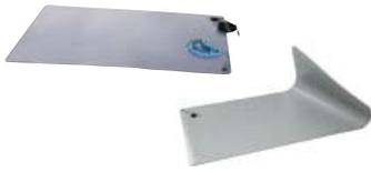
LABESTAT mats are made from a rugged synthetic rubber resistant to hot solder, fluxes and chemicals. The underside layer is black conductive, the top grey layer, glare free surface, has a resistance from  $10^7$  to  $10^9 \Omega$ .
